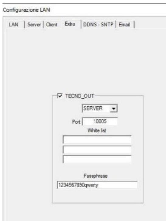
The screenshot shows the 'Configurazione LAN' window with the 'Server' tab selected. The 'TECNO\_OUT' protocol is enabled (checked). The configuration includes a dropdown menu set to 'SERVER', a 'Port' field with the value '10005', a 'White list' section with three empty input fields, and a 'Passphrase' field containing the text '1234567890qwerty'.
